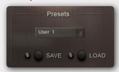
To save your user settings as a preset, Go to: Option\Performance\Presets section, select one of the drop-down menu's 10 empty presets and press the SAVE button. To load the presets choose a Preset on the drop-down menu and press the LOAD button.
